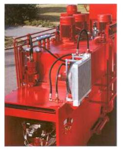
The compact hydraulic system has low-noise drives, an automatic pump-demand control as well as minimal hydraulic piping. This guarantees low energy and maintenance costs.
