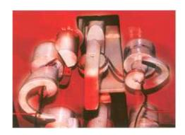
The fully automatic tying system has an integrated cutting device, making it highly efficient and reliable even during heavy-duty operation. Short wire end ties ensure that the minimum of wire is used and make the Konti E-series even more cost effective.
