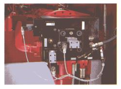
PAAL developed and patented the hydrological block. Mounted directly onto the hydraulic cylinder, this helps to minimise heat generation and energy losses.
