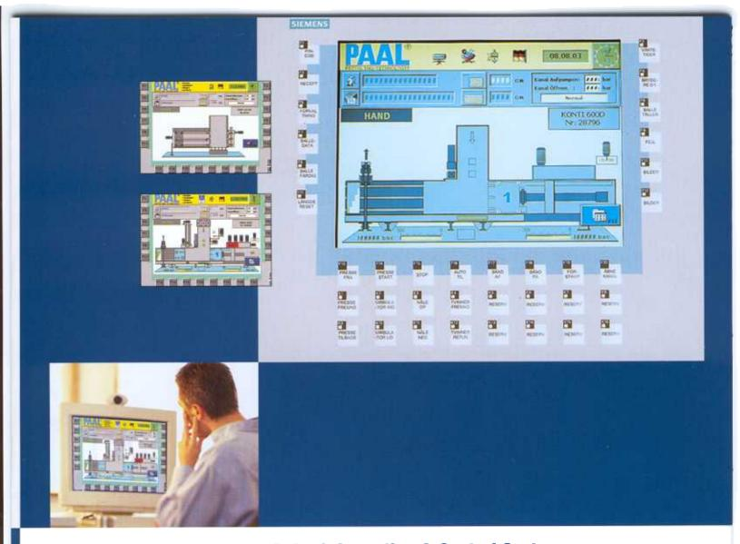
With the integrated modem we are able to contact the machine plc and thus when "online" react to and rectify malfunctions.
